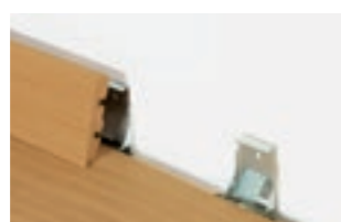
Wallbase installation clips PGCLIPSKME95 – modern plank 9 mm PGCLIPSKME7080 – domestic elegance For PGSK(-) wallbases only. Easy-to-use snap-in system where no nails or screws are needed. One installation kit covers 20 metres of wallbase.
