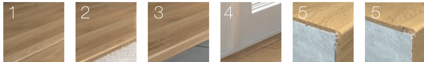
1 T-moulding From wood to wood. 2 Carpet transition From wood to carpet. 3 Hard surface reducer From wood to ceramic, vinyl or linoleum. 4 End moulding Finishing up to threshold, sliding doors, etc. 5 Stair nose moulding, flush For a flush finish on stair treads. 5 Stair nose moulding For a step down from a floating floor, e.g. at the top of the stairs or a step down in a room.
